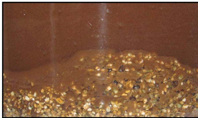
Figure 5-6. Photograph of the chabazite-SBR during the aerobic stage showing zeolite material settling despite mixing.
